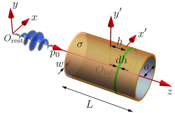
FIG. 1. System in which an electron vortex beam with a central energy  $\mathcal{E}$  and momentum  $p_0$ , which is in its lower longitudinal mode  $[u_{p,\ell}^{\text{LG}}(r, \varphi; t) u_n^{\text{HG}}(\zeta) e^{i(p_0 z - \mathcal{E}t)/\hbar}]$ , propagates through a cylinder with conductivity  $\sigma$  and permeability  $\mu$ . The relative motion of both entities results in the generation of a current in the infinitesimal loop of thickness  $dh$ .
